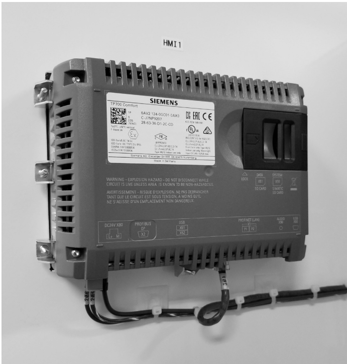
Figure 2.3.1b Rear view of HMI.
