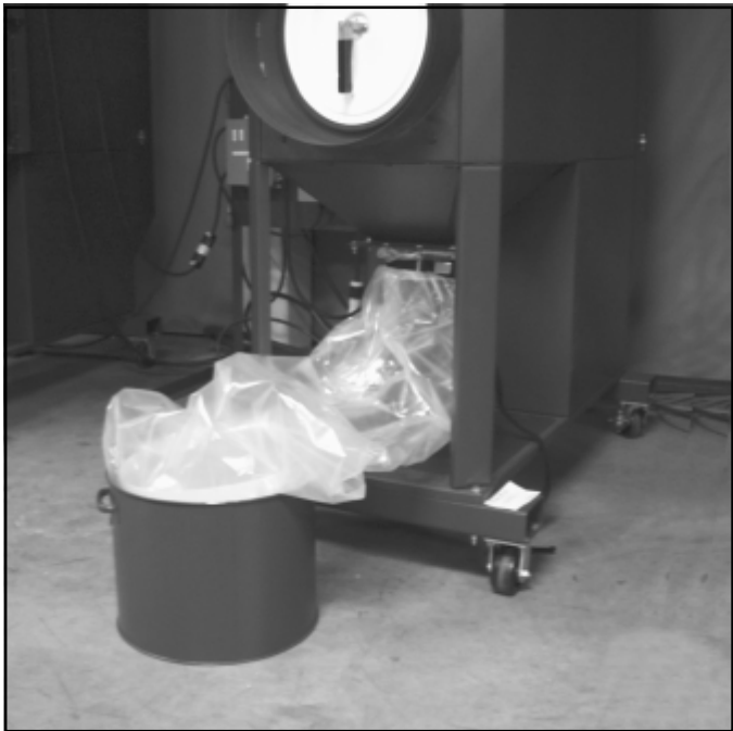
Secure Bag to Collar Adapter With One Safety Strap
