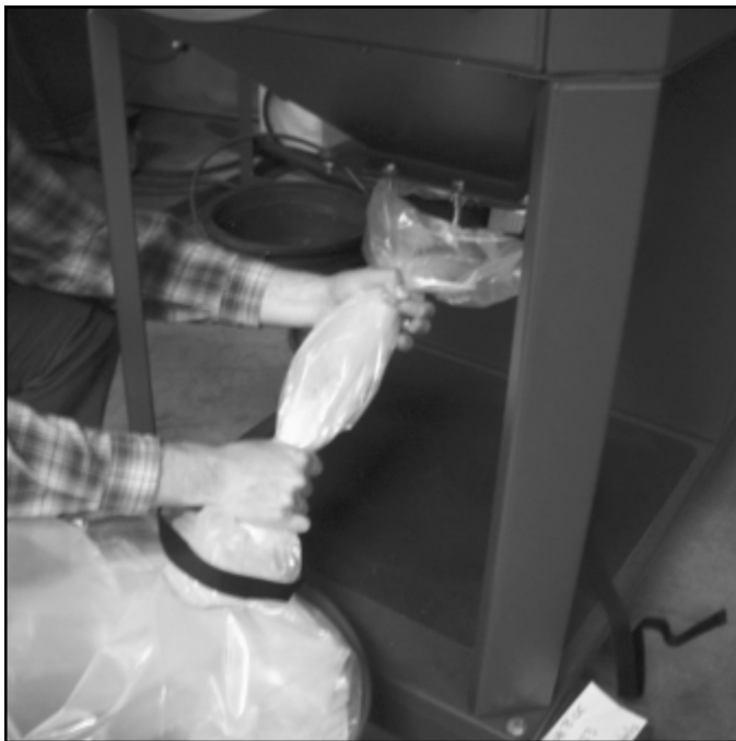
Seal the Bag Using Two Cable Ties
