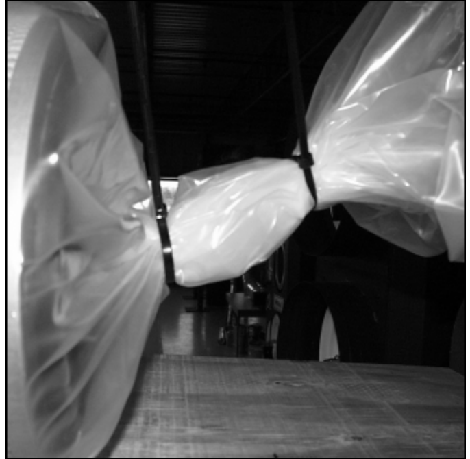
Cut Between Cable Ties
