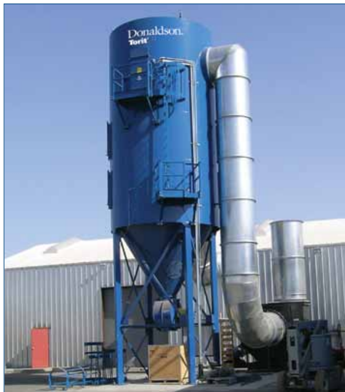
The Dura-Life bag filters in this Donaldson Torit RF Baghouse collector provide longer life and lower emissions at this Midwestern soybean processing plant.
