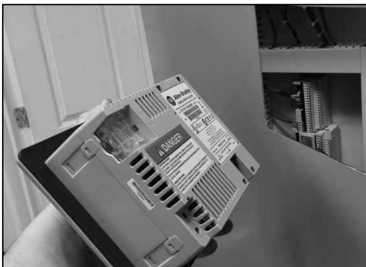
Figure 2.3.9: HMI, completely removed
