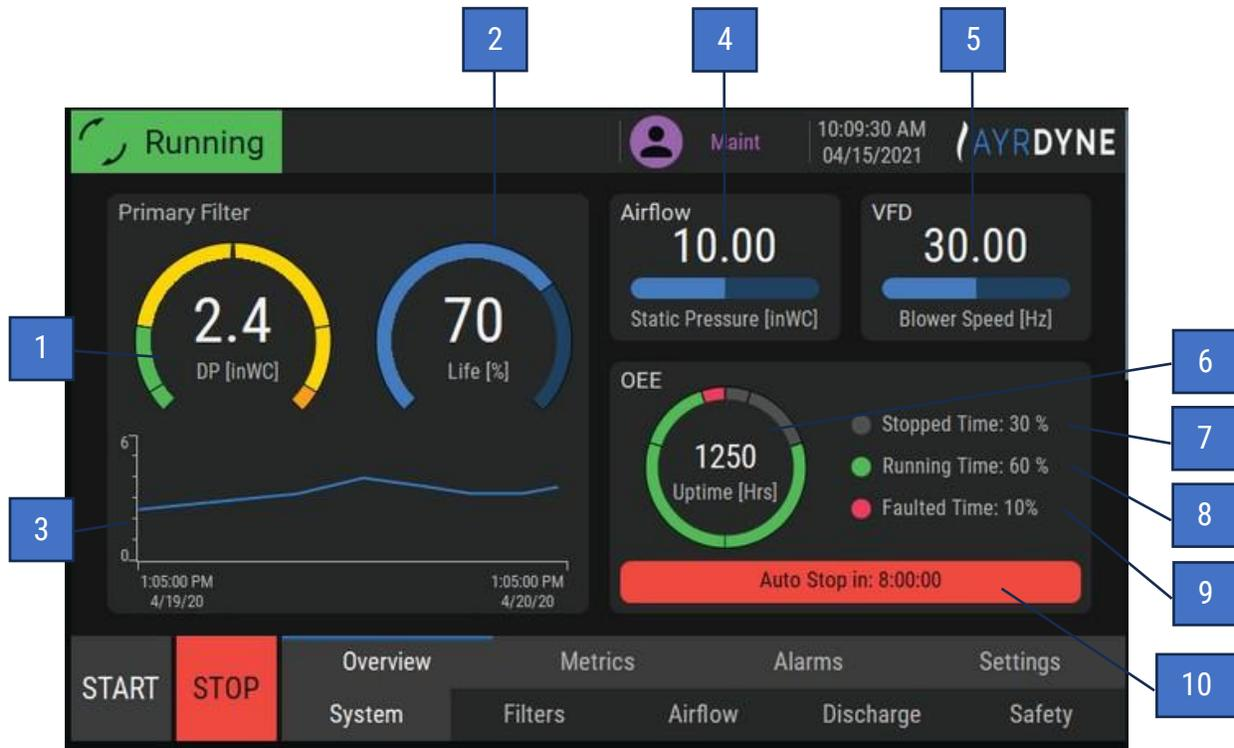
**1. Primary filter DP** – This numeric display and dial display show the filtered differential pressure measured between the dirty and clean sides of filters.
