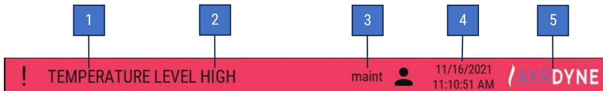
The status bar is visible on all screens. This bar displays system information, active alarm description, and corrective action.
