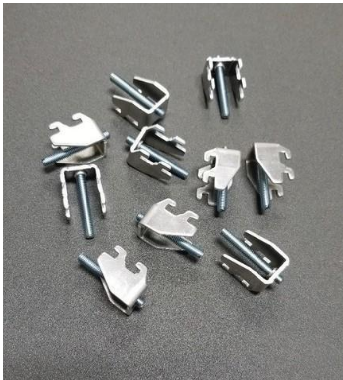
Figure 4 Installation fasteners removed
