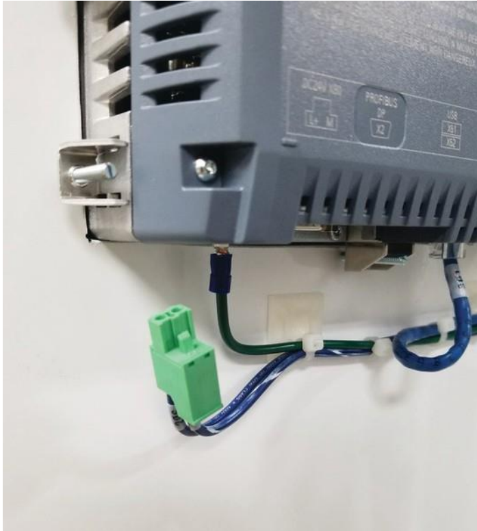
Figure 1 Power connection removed from HMI
