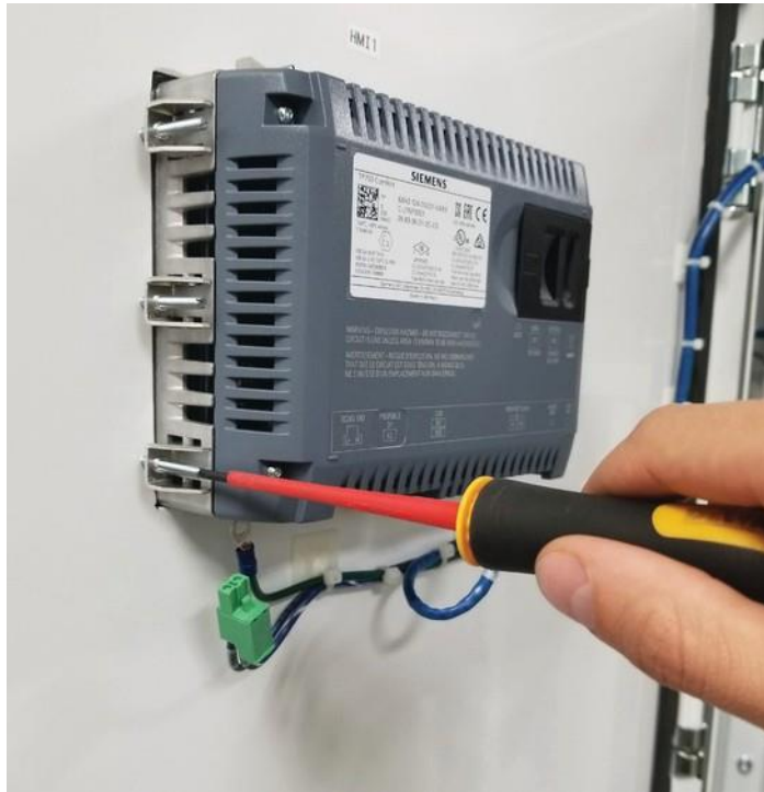
Figure 3 Loosening HMI fasteners
