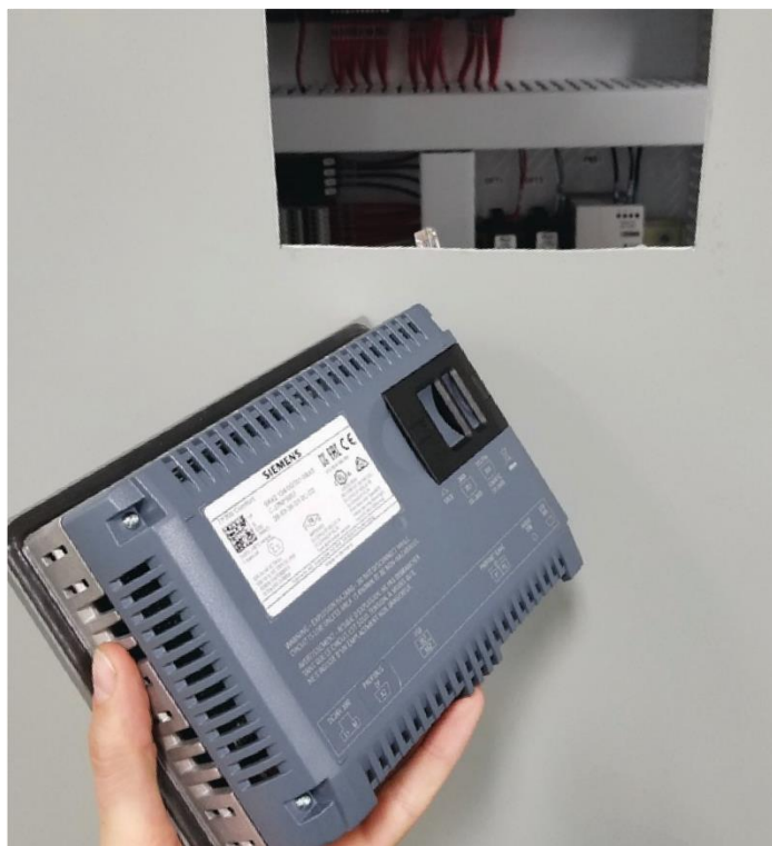
Figure 6 HMI completely removed
